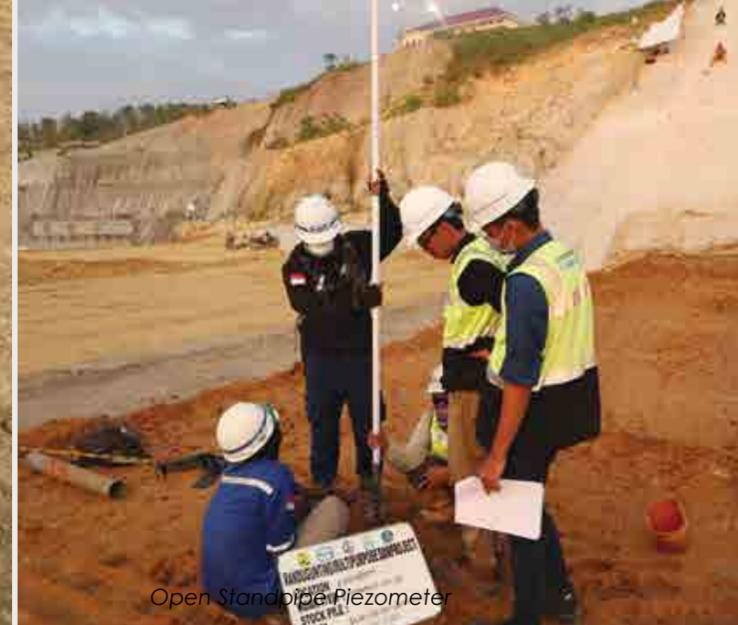
Open Standpipe Piezometer
